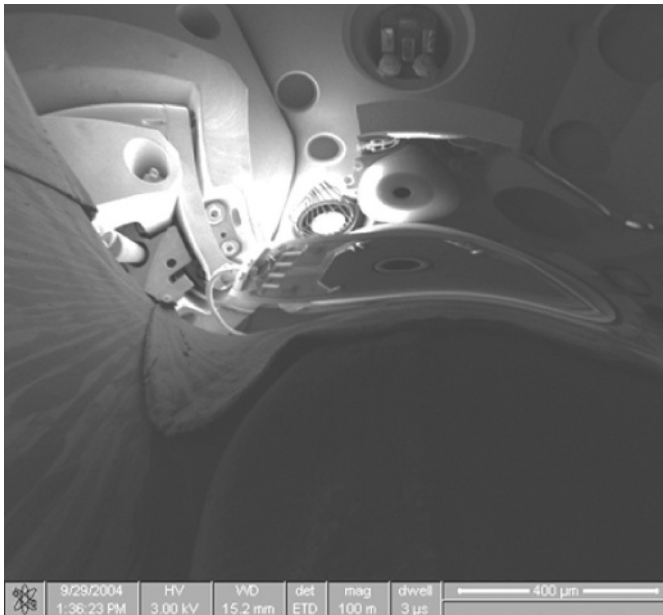
Figure 1.2 The ‘mirror effect’. Instead of landing on the specimen and forming an image of the specimen surface, primary electrons are repelled by the electric field arising from electrons implanted in the specimen, and turn back to strike the lens and other parts of the microscope. This generates signals that form an image of the inside of the chamber (distorted in this case)
